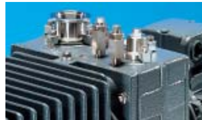
Sensors connections on 2033C2
